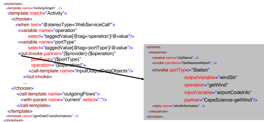
Figure 4 From XMI Light to a BPEL4WS document using XSLT
